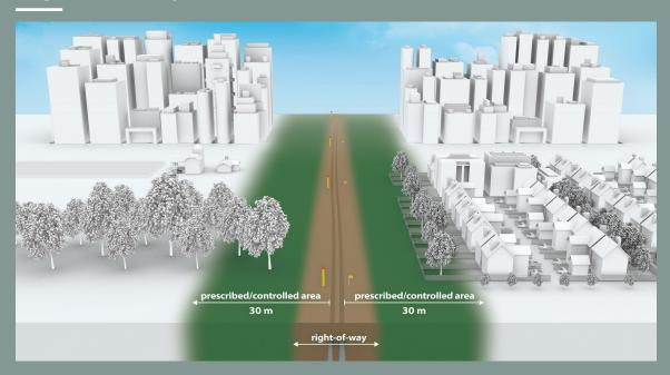
A pipeline right-of-way (ROW) is the strip of land where the pipeline is located. The width of the ROW may vary depending on factors such as pipeline diameter or the number of pipelines in an area. The area extending 30 meters (100 feet) on either side of the pipeline is called the Prescribed Area / Controlled Area.
